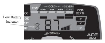
The Low Battery Indicator will switch on when the detector's batteries become weak. The detector will maintain full performance but the batteries should be replaced soon when this indicator appears. NiMH rechargeable batteries may be used, but may have a shorter life per charge. You can expect 20 to 40 hours of operation depending on battery type and quality.
