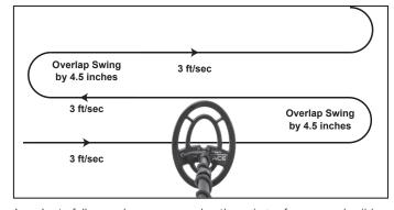
In order to fully search an area, overlap the swings of your searchcoil by half the length of the coil (about 4.5 inches). Sweep the searchcoil in a straight line or with a slight arc at a sweep speed of about 3 ft/sec.
