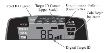
**Target ID Legend**—Works with the Target ID Cursor to indicate a target's probable identity, with Ferrous (iron) targets at the left, non-ferrous targets that are thin or have low conductivity in the middle, and thick or high conductivity targets (e.g. thick silver) at the right.
